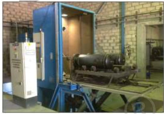
SPL. PRESSURE BLASTER MACHINE CYLINDER ID CLEANING
