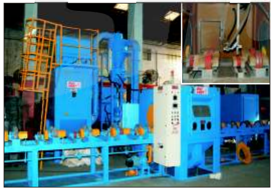
SPL. BLASTING MACHINE TO BLAST CLEAN BOILERS TUBES
