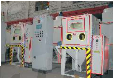
SPL. BLASTING M/C TO BLAST CLEAN GEAR CUTTING TOOLS BEFORE PVD COATING
