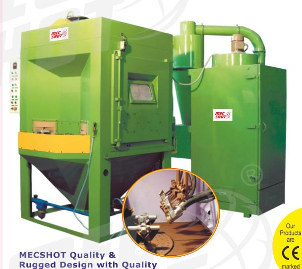
MECSHOT has developed an equipment to descale, surface preparation and other finishing application on automotive component like gears, shafts, camshafts, spiders, brake shoe, piston head etc. The Machine operates on the suction principle of abrasive blasting.
