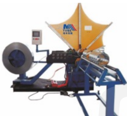
Tubler Duct Manufacturing M/c
