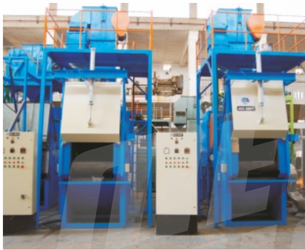
ATB 27" x 36" with Pneumatic Control Door
