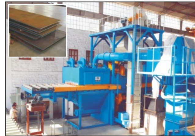
Tunnel Type 4 Wheel Shot Blasting M/c for Heavy Plate Cleaning
