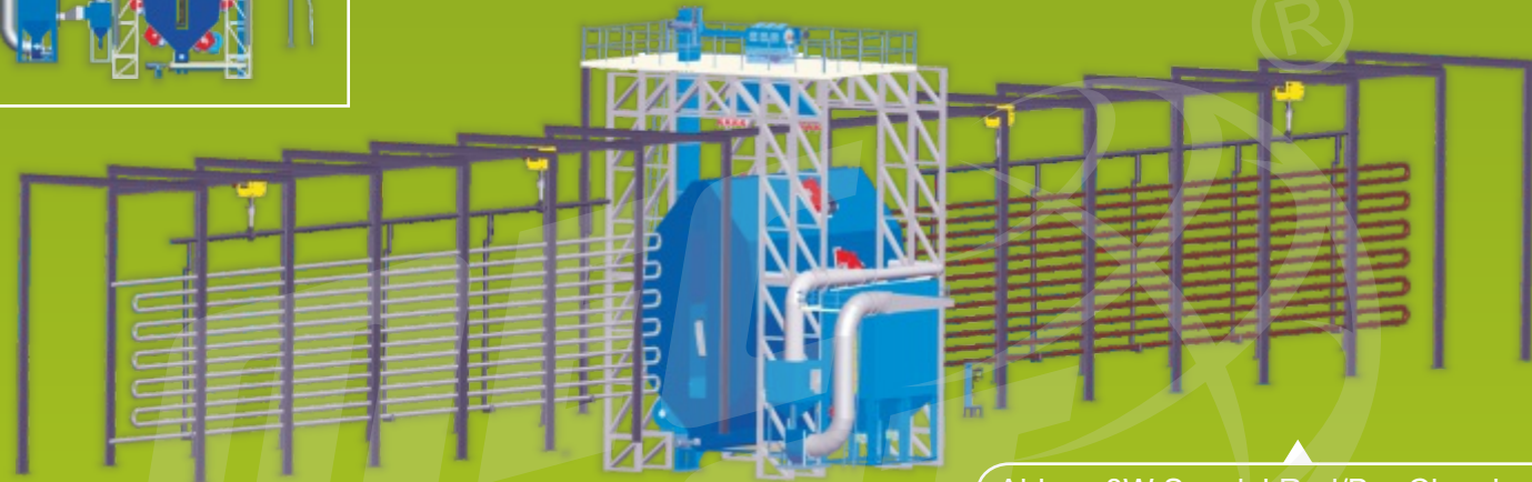
Airless 8W Special Rod/Bar Cleaning M/c
