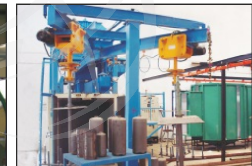
'Y' Hanger Type Shot Blasting M/c for Fire Extinguisher Cylinder
