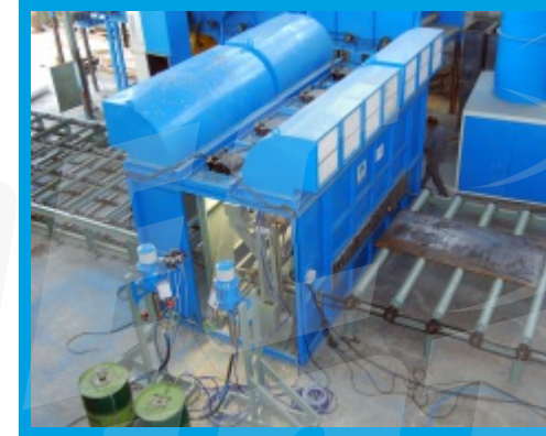
PAINT SPRAY BOOTH WITH WIWA PAINTING EQUIPMENT
