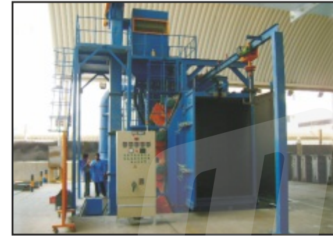
'T' Hanger Type Shot Blasting M/c with Motorized Hoist for Electric Transformers
