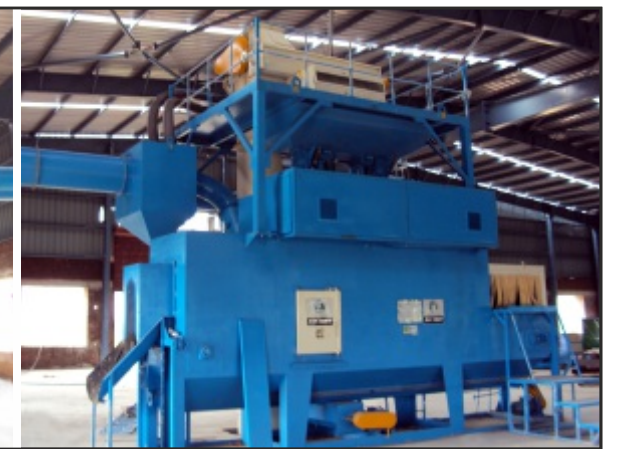
Airless 2 Wheel Shot Peening M/c With Airless Magna Valve for Coil Spring Dia 50 to 500 mm
