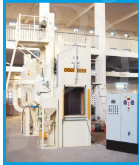
Airless Shot Blasting M/c with Indexing Hanger for Automobile Components
