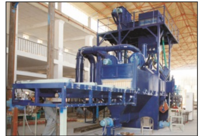
Tunnel Type 6 Wheel Shot Blasting M/c for Plate Cleaning before Painting
