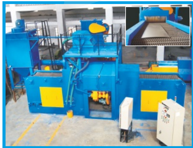
Airless 2W Metallic Conveyor Type Shot Blasting M/c for Iron Plate / Marble / Granite etc.
