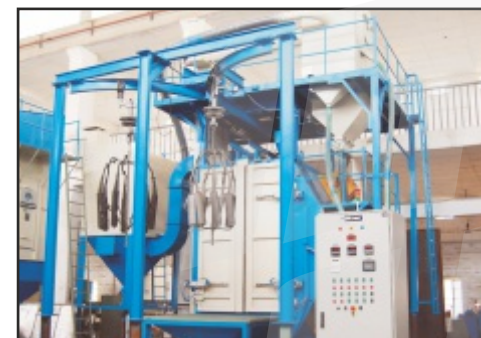
'Y' Hanger Type Shot Blasting M/c for Automobile Mufflers
