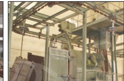
Continuous Monorail Hanger Loop Type Shot Blasting M/c for Electric Transformers
