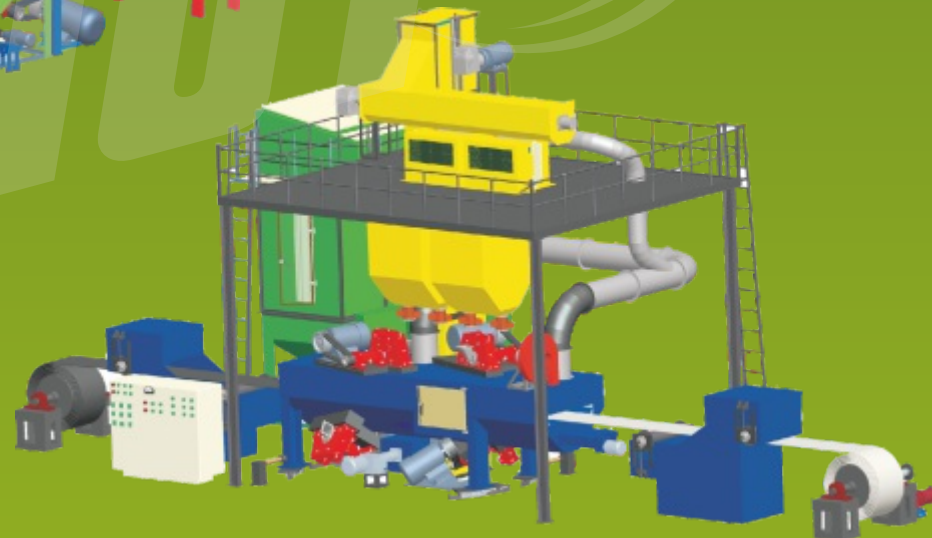
Airless 4W Special Strip Cleaning M/c
