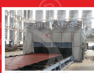
Paint Spray Booth
