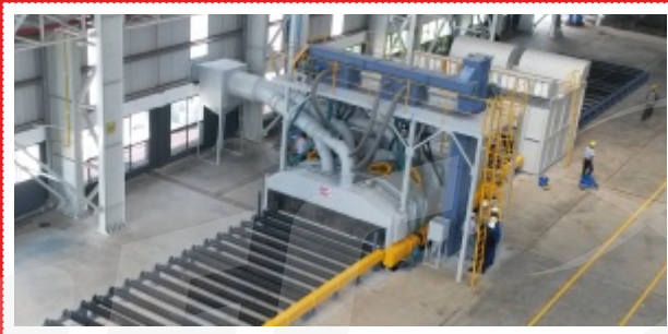
Airless 4 Rotor Type Blasting M/c with Pre Heating Chamber for Plate Cleaning
