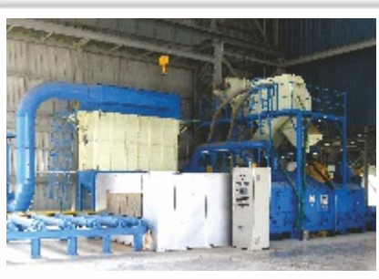
Airless 4 Rotor Type Blasting M/c with Pre Heating Chamber for Plate Cleaning
