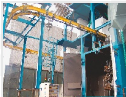
Continuous Loop Hanger Type Blasting M/c for Automobile Engine Cylinders
