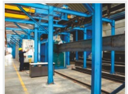
Continuous Loop Hanger Type Blasting M/c for Structures
