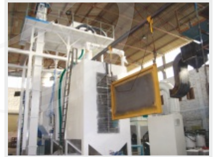
'T' Hanger Type Shot Blasting M/c for Tipper & Trailer Industry
