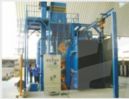
'T' Hanger Type Shot Blasting M/c for Electric Transformer Industry
