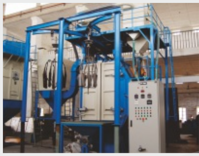
'Y' Hanger Type Shot Blasting M/c for Automobile Mufflers
