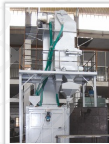
Airless 2W Hanger Type Blasting M/c for Automobile Industry with Magnetic Shot Separator
